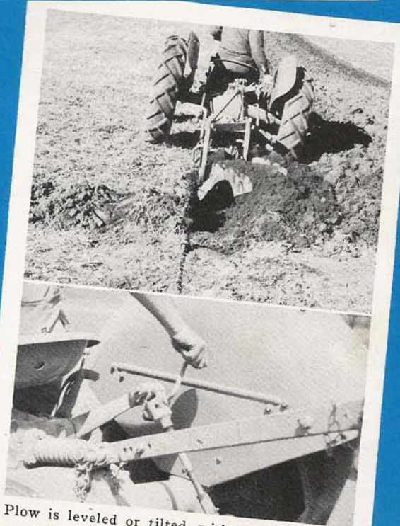
Full-width furrows, straight from one end of the field to the other, are made by keeping right tractor wheels against the furrow wall.
