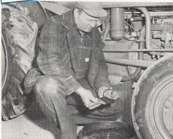
Clean oil pump screen (on drain plug) in gasoline at each oil change. Replace carefully.
