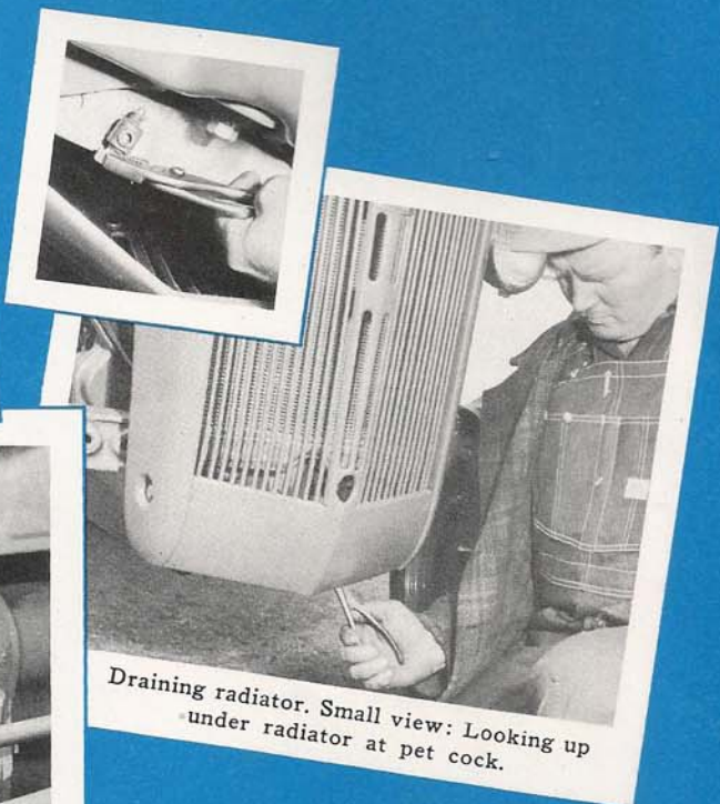
Radiator water must be clean. If it causes rust, add a rust inhibitor.
