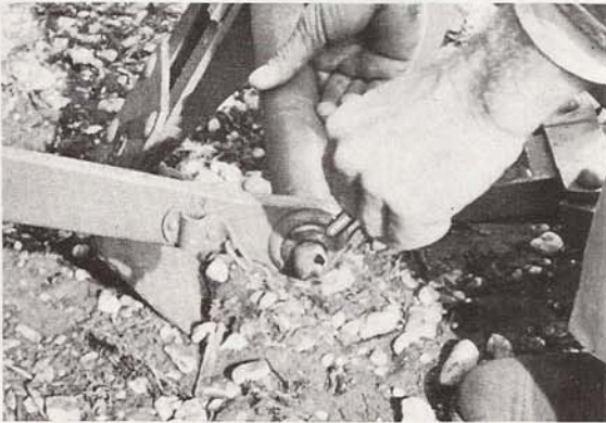
Attaching disc harrow. (1) Lower linkage with finger tip control lever, then attach lower left link.
