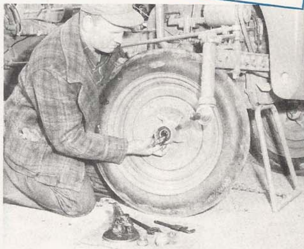
Four Lubrication Rules: (3) Repack front wheels with short fiber grease once each season.
