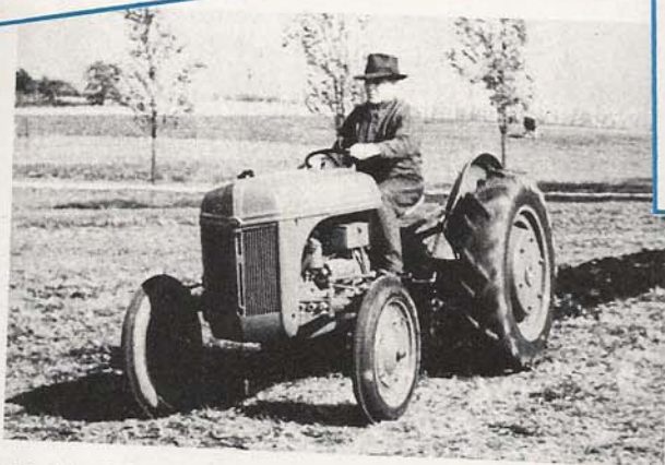
Headland furrow. Use rear base only. Plow 2" to 4" deep.
