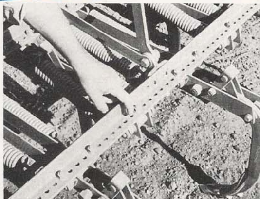
Tines may be spaced by 1" intervals to suit different requirements.
