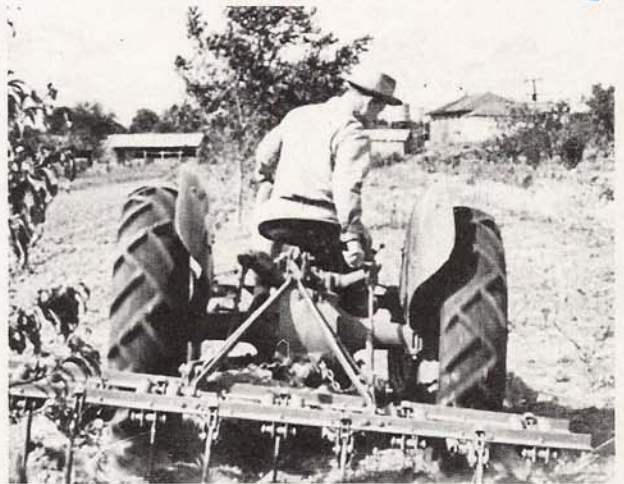
Tiller can be tilted with leveling crank when working in orchards close to trees.
