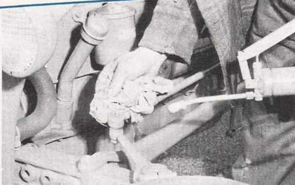
Four Lubrication Rules: (1) Keep nine fittings lubricated with grease gun.
