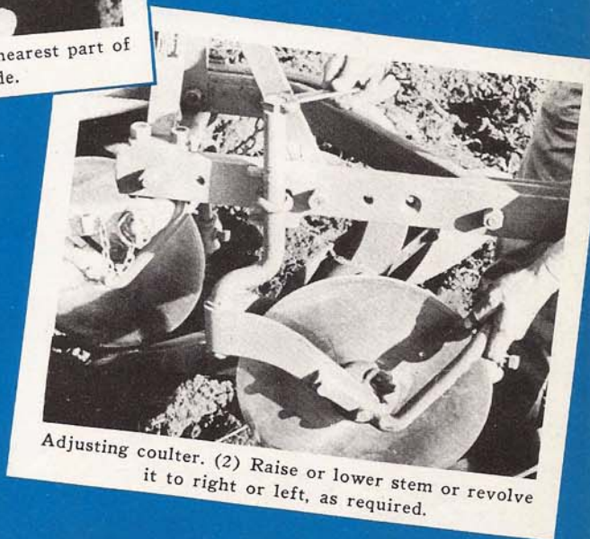
Adjusting coulters. (1) Loosen eyebolt that holds stem.
