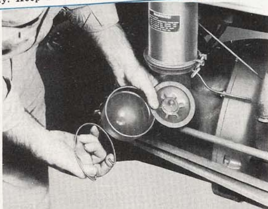
Showing the three parts of the oil cup assembly.
