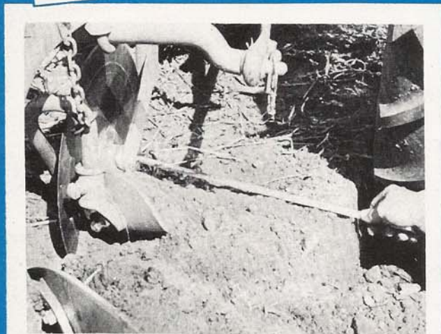
Width of cut is measured from furrow wall to front coulters.
