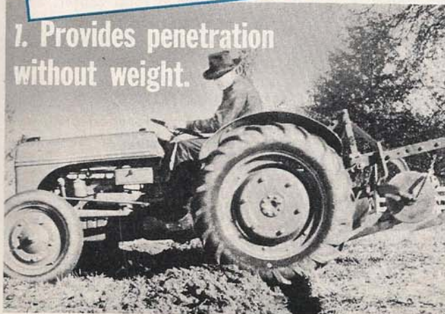
About to lower plow. Ferguson System provides penetration without excess weight.
