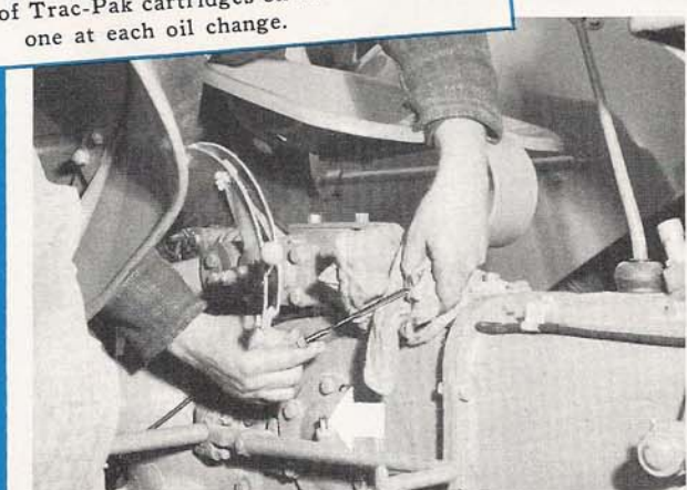
The same lubricant is used in transmission, differential and hydraulic. Change after first 200 working hours; thereafter, each 600 hours.
