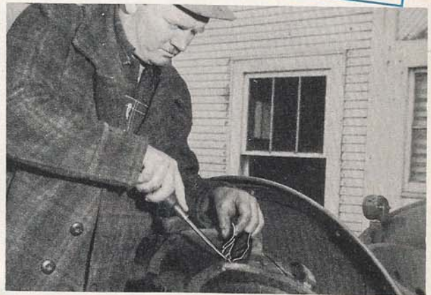
Clean cracks in tires with gasoline and fill with gum rubber made for the purpose.
