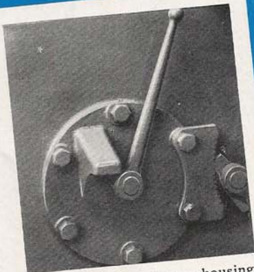
Lever, on left of center housing, engages and disengages power take-off and hydraulic pump.
