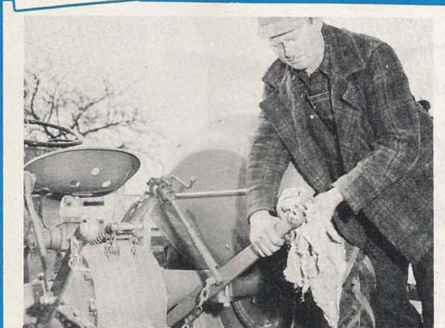
To keep linkage working smoothly, wipe ball joints and connections, but do not lubricate.
